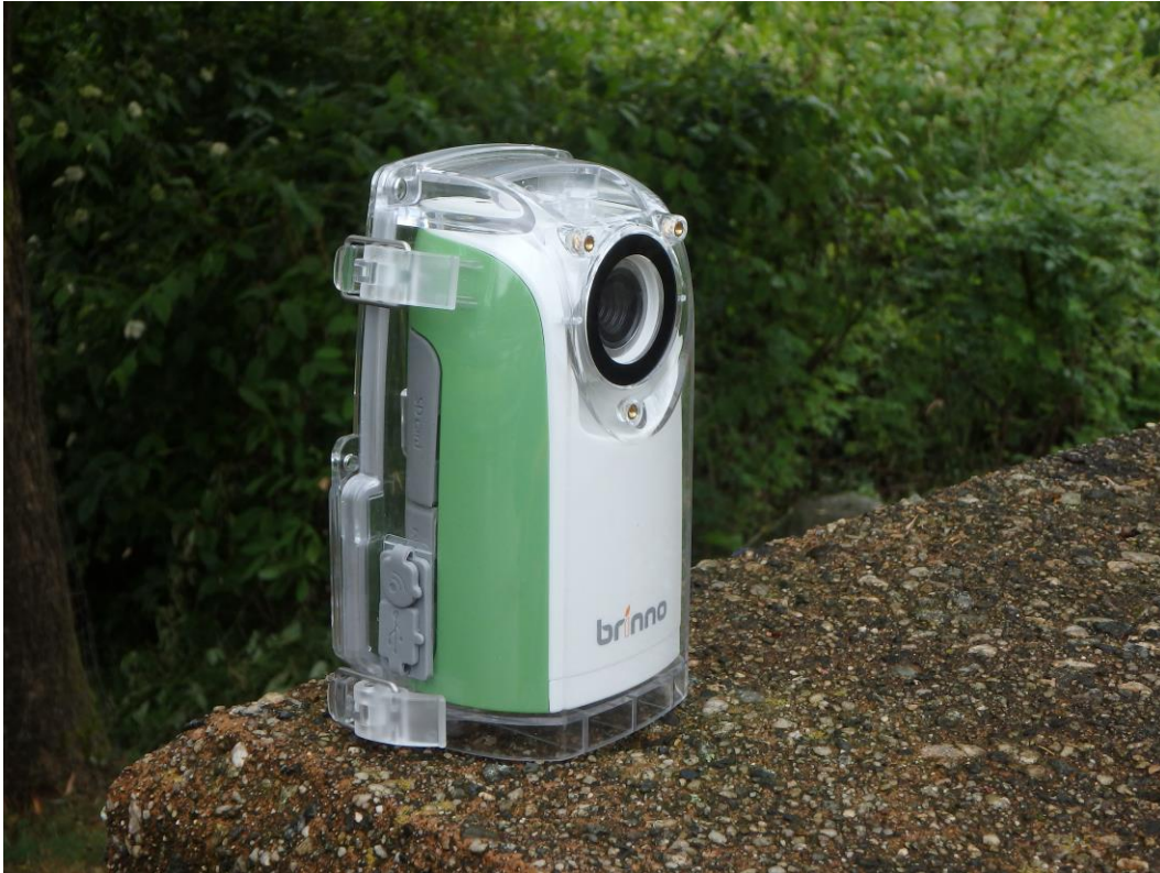
Figure A1. Brinno TLC200 time-lapse camera in weatherproof housing
