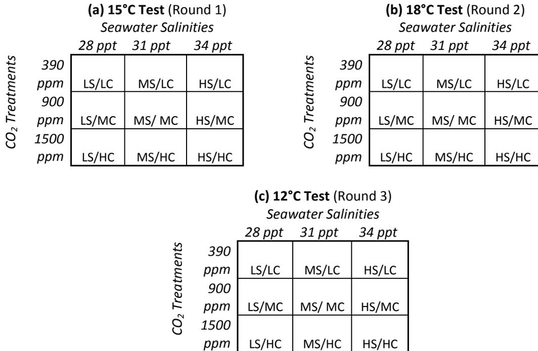
Figure 3. Test Treatment Schematic. Nine treatments consisting of combinations of salinity and CO<sub>2</sub> stressors were set up at (a) 15°C (Round 1), (b) 18°C (Round 2) and (c) 12°C (Round 3), for a total of 27 treatments.
