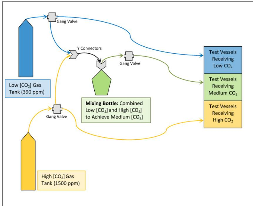
Figure 2. CO<sub>2</sub> tank and mixing bottle schematic. The medium CO<sub>2</sub> concentration was prepared by mixing the high and low CO<sub>2</sub> gases through a mixing bottle.
