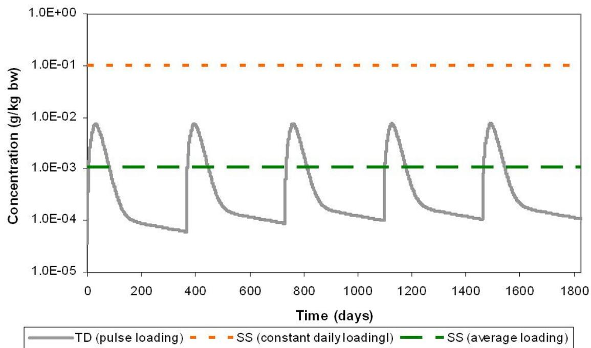
**Figure 4-27** Comparison between steady-state and time-dependent bioaccumulation model predictions of metaflumizone concentrations in forage fish B. TD (pulse loading) represents time-dependent model predictions with application rate of 14g/application at 7-day intervals; SS(constant daily loading) represents steady-state model predictions with daily loading of 14g of metaflumizone; SS(average loading) represents steady-state model predictions with daily loading of 0.1534g of metaflumizone.
