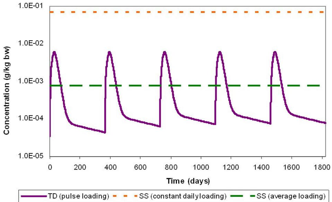
**Figure 4-26** Comparison between steady-state and time-dependent bioaccumulation model predictions of metaflumizone concentrations in forage fish A. TD (pulse loading) represents time-dependent model predictions with application rate of 14g/application at 7-day intervals; SS(constant daily loading) represents steady-state model predictions with daily loading of 14g of metaflumizone; SS(average loading) represents steady-state model predictions with daily loading of 0.1534g of metaflumizone.
