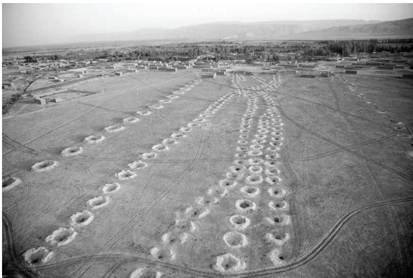
Figure 3. A bird's eye view of the karez system in the Turpan Oasis (photo courtesy of Geroge Steinmetz).
