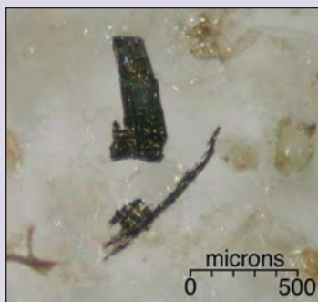
Figure 3. Photograph of two charcoal fragments isolated from lake sediment by wet sieving and retaining the 125–250 \mu\text{m} size class. Charcoal records are usually based upon time series of charcoal quantity from lake sediment or other stratigraphic sequences. This sediment sample was treated with weak hydrogen peroxide, causing non-charcoal organic material to become almost translucent.
