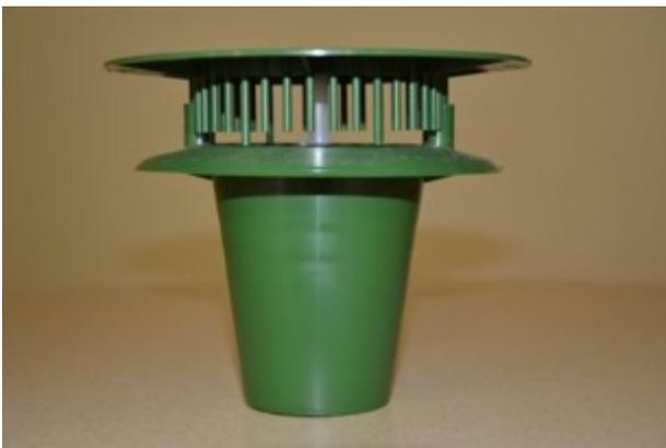
**Plate 1.1. The trap designed by R. Vernon has small pins extending down from the lid to allow invertebrates in but to exclude small mammals or rodents**
